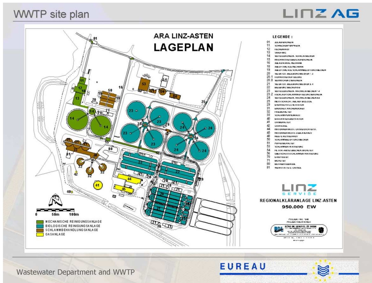
Figure 2: Map of WWTP Linz with the two primary clarifiers in green and indicated with No. 14
