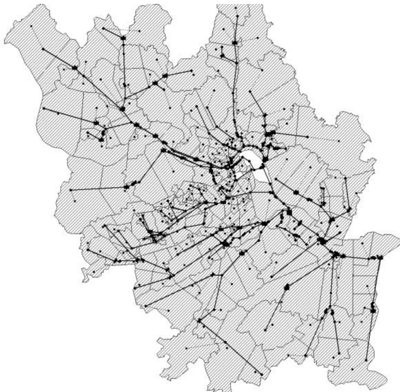
Figure 1: Overview of aggregated Linz catchment model in SWMM 5 (Gamerith et al., submitted)
