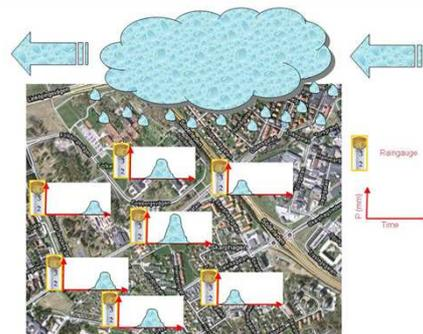
Figure 2. Schematic of the storm generator, simulating the passage of a storm over a catchment and generating consistent time series (design storms) in selected locations.
